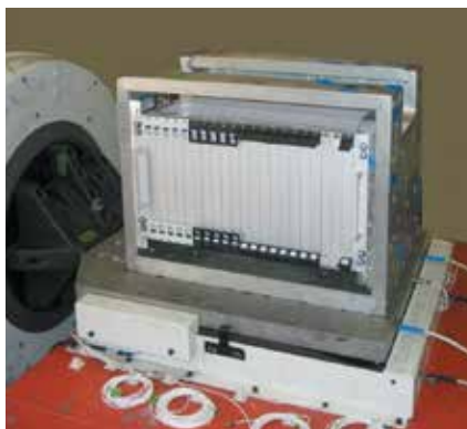
Illustration: Shock and vibration test to MIL 810G and IEC 61587-1, requirement classes DL2 and DL3
