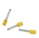
The single wire DIN end sleeve insulated ferrule has a funnel entry for faster insertion and lower installation cost. It is intended for American Wire Gauge (AWG) #16 (1.5 mm<sup>2</sup>) wire ferrules and supports a maximum wire insulated diameter of 0.12" (3.0 mm).
