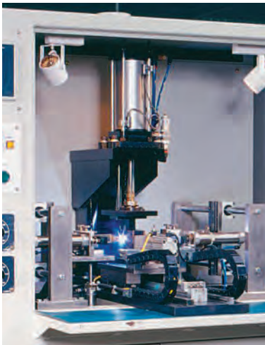
High-speed automated welding equipment for transformer cores provides economical production.
