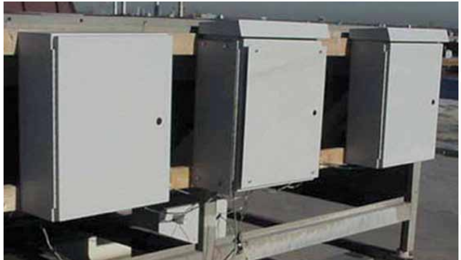
Illustration of the test set-up. The enclosures used were Hoffman COMLINE® model E-CL605020 (600mm H X 500mm W x 200mm D). They are RAL 7035 (Textured Light Gray) in finish and color. The top solar shield is model E-SSH5020.
