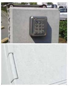
Prolonged UV exposure can cause fiberbloom on fiberglass enclosures, a form of surface degradation that results in loss of color and gloss.
