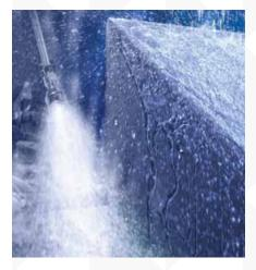
While some enclosures are specifically built to protect against washdown, high-pressure spray may penetrate around sealed components and gaskets in many enclosures.
