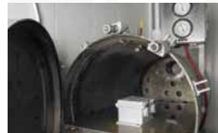
Type 6, 6P Water Submersion Test
