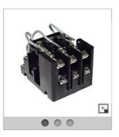
The 425 3 pole relay is capable of handling up to 30 Amp and 1HP loads. The 425 series (3 pole) has sufficient spacing to allow for 600VAC contact rating. The design features an enclosed coil, screw terminals, and silver alloy contacts as standard. The 425 has a wide choice of options to choose from.
