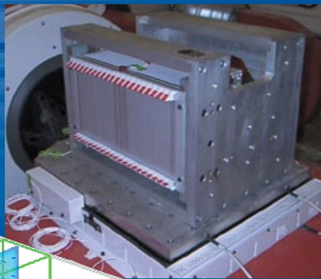
Subrack shock and vibration test
