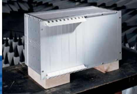
Subrack electromagnetic shielding performance test
