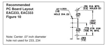
Note: Unless otherwise specified, all dimension tolerances are  $\pm$  .01 inch (+0.25 mm)
