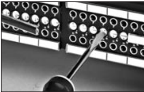
Center Strip Removes For Normaling Access
