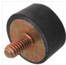
Single End Male Sandwich Mount: 50 lbs (22.7 kg) Compression Load, 1/4-20 Threads, 1.000 in (25.4 mm) Base Diameter
