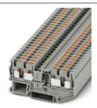
Component terminal block, with integrated diode, Connection method: Push-in connection, Cross section: 0.2 mm<sup>2</sup> - 6 mm<sup>2</sup>, AWG: 24 - 10, Width: 6.2 mm, Color: gray, Mounting type: NS 35/7,5, NS 35/15
