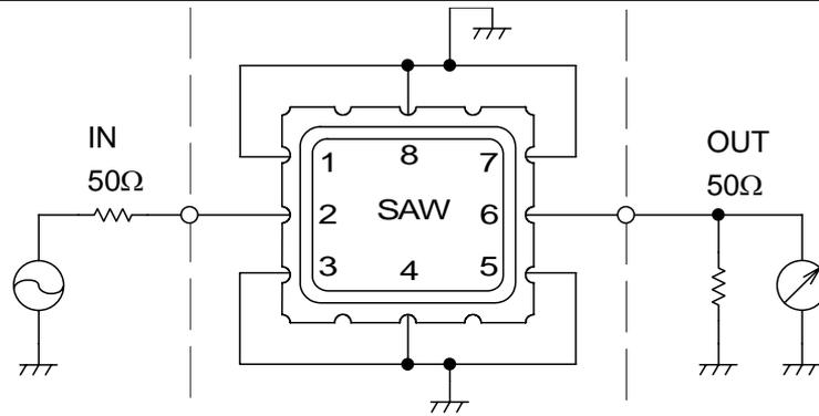
Fig.1 Measuring circuit
