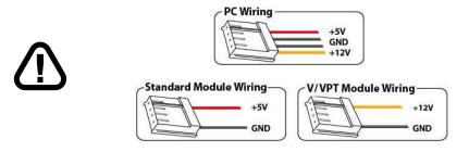
Figure 11: PC vs Matrix Orbital Display Module Wiring
