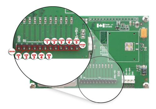
Figure 21: Keypad Interface Connector
