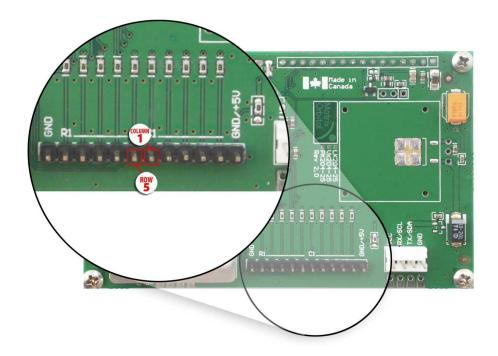
Figure 20: Manual Override Jumper
