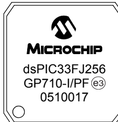
100-Lead TQFP (14x14x1mm)
