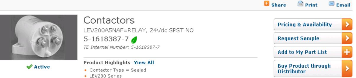
Contact - Arrangement = 1 Form A, SPST-NO Documents Features Compliance Please Note: Use the Product Drawing for all design activity **Contact Features** Product Type Features **Contactor Type** Sealed Number of Poles 📳 1 Terminal Configuration 10-32 Stud **Configuration Features Electrical Characteristics** Contact - Arrangement 1 Form A, SPST-NO Actuating System ? DC Cont Coil (VDC Coil
