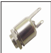
30-624-2.1 30-624-2.5 Chassis mount locking DC power coax jack. Mates with 30-623 plug. Mounts in panels up to .07".
