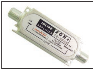
75-725 16-20dB SLOPED 950-2250MHz amplifier High quality satellite RF inline amplifier suitable for DBS or MMDS satellite applications. Sloped gain for long cable runs. Epoxy sealed back cover plate. Power requirements 12-18Vdc, 45mA. DC pass through current 500mA maximum. Output level 105dBuV maximum. Low noise 5dB - input return loss 6dB. Impedance 75 ohms - frequency 40-2250MHz. High performance SMD board circuitry. Precision machined F-connector threads. Nickel plated zinc alloy diecast housing.
