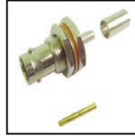
75-685 BNC Female chassis mount jack for RG-174U cable. 75 ohm. Fits in a 1/2" "D" hole. Bushing length .33"
