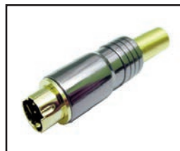
30-505 (4 pin) 30-505-6 (6 pin) 30-505-8 (8 pin) Pro quality Mini Din connector for 5-7mm cable. Metal housing with gold pins, contacts and strain relief. .27" cable opening.
