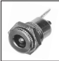
30-379 3.0mm I.D. 6.3mm O.D. chassis mount coax power jack. For \frac{7}{16} " dia. hole in panels up to \frac{3}{16} " thick.
