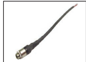
30-493A-6 inch 3.5mm Mini stereo audio jack with 6 inches stripped and tinned leads. Shielded two conductor cable with Black shrink tube strain relief. Red and Black wire color. Mounts in 1/4 hole. .165" bushing length.
