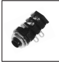
30-395 Open Circuit. 30-396 1/4" Audio Jack. Closed Circuit 2-Conductor. 3/8" bushing. Mounts in .355" hole.
