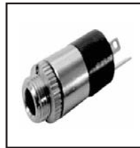
30-493A, 3.5mm 30-494A, 2.5mm Mini or sub mini stereo Audio Jack. Panel mount. Mounts in .25 hole. Bushing length .165".
