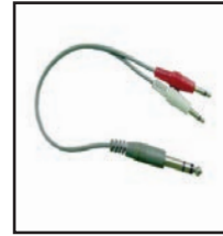
35-533 Stereo 1/4" plug to two 3.5mm mono plugs, shielded. 11" long.
