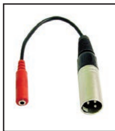
35-469 3.5mm stereo Female jack to XLR Male plug. Wired: pin 1 = ground pin 2 = tip pin 3 = ring. 8" long. Black PVC jacket.
