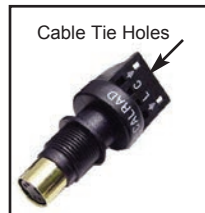
35-498k-s Solderless Keystone & Chassis Mount SVHS Jack. Easily mountable SHVS jack for either 1/2" chassis mount or keystone insert. Screw terminals provide a clean, solderless, connectorless backside termination. Includes colored cable tie for strain relief. Colored plastic washer available for enhanced visual ID (Part Number 30-288-Color).
