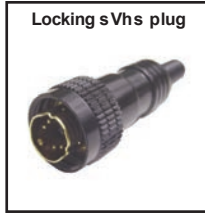
30-505-Lk Locking 4 pin SVHS Male connector. Spring strain relief, Black. Mates with 30-507 chassis mount jack.
