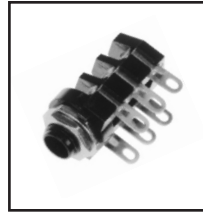
30-399 1/4" Audio Jack. 3-Circuit, 3 Closed. 3/8" bushing. Mounts in .355" hole.
