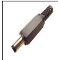
30-635 Coax AC/DC power plug 4.75mm O.D., 1.7mm I.D., 9.2mm long, .17" cable opening. 30-632 same as 30-635 with O.D. of 4mm.
