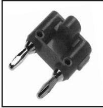
30-440-Nk Red 30-441-Nk Black Dual banana plug, nickel plated. .24" cable opening. 0.75" centers.
