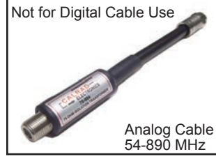
75-504 DC GROUND BLOCKER & ISOLATION trAnsformer 75 ohm In/Out, Male 'F' connector to Female 'F' connector. Eliminates hum bars or audible hum generated when A/V components are connected directly to a cable TV or satellite system. Isolates ground potential differences within an Audio/Video system without affecting the RF signal. Frequency range 54-890MHz. 6" long.
