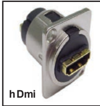
35-723 'D' Style panel mount HDMI female-panel female feed-thru. Gold plated contacts. Mounts in a .917" hole.
