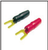
30-613-Bk Black 30-613-RD Red 30-613 Red&Black Spade terminal, gold plated crimp on connector, with P.V.C. cover, black or red. .15" to .3" cable opening.
