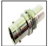
75-521-3/8 Panel feed thru connector. BNC Female to RCA Female. Bushing dia.: .365" Bushing length: .27" Overall length is 1.06" Mounts in .375" hole.
