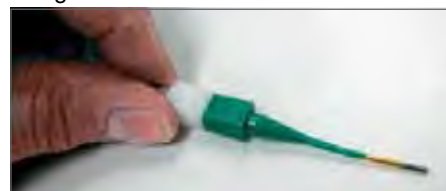
Plastic tool with contact in proper position.
