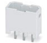
Header, Nominal current: 6 A, Rated voltage (III/2): 160 V, Number of positions: 8, Pitch: 2.5 mm, Color: white, Contact surface: Tin, Mounting: THR soldering
