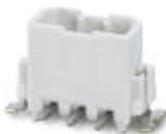
Header, Nominal current: 6 A, Rated voltage (III/2): 160 V, Number of positions: 8, Pitch: 2.5 mm, Color: white, Contact surface: Tin, Mounting: SMD soldering, Article with anti-rotation pin
