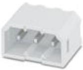
Header, Nominal current: 6 A, Rated voltage (III/2): 160 V, Number of positions: 8, Pitch: 2.5 mm, Color: white, Contact surface: Tin, Mounting: THR soldering
