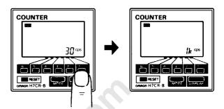
Press the DISPLAY key to return to RUN mode from SETTING mode.
