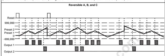
**Output Mode D** Present value increments and decrements within displayable range. Output 1 is ON whenever present value is equal to preset 1; Output 2 is ON whenever present value is equal to preset 2.
