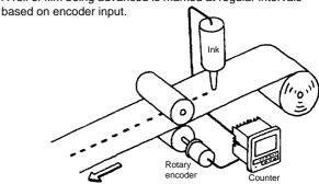
Choose Mode P to put the count-up value on hold (display is on hold while the one-shot output is ON). There is no difference in operation between Mode C and Mode P.
