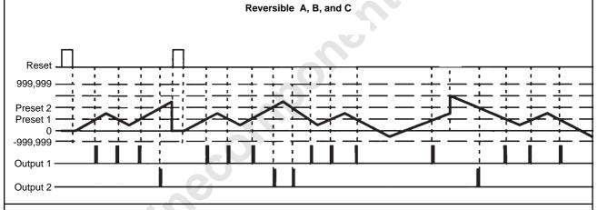
**Output Mode L** Present value increments and decrements within displayable range. Output 1 is ON whenever present value is less than or equal to preset 1; Output 2 is ON whenever present value is greater than or equal to preset 2.
