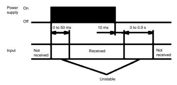
For 100 to 240 VAC and 24 VAC/12 to 24 VDC counters, be sure that the capacity of the external power supply is adequate, because the power supply may not provide a surge current sufficient to start the counter due to the switching regulator contained in the counter's internal circuitry.
