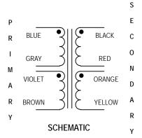
Primary and secondary windings are designed to be connected in series or parallel. Windings are not intended to be used independently.
