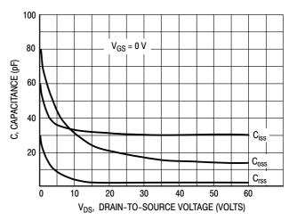
Figure 6. Capacitance versus Drain-To-Source Voltage
