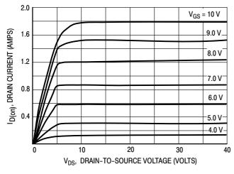
Figure 5. Output Characteristics
