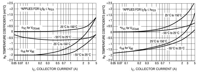
**Figure 7. Temperature Coefficients**
