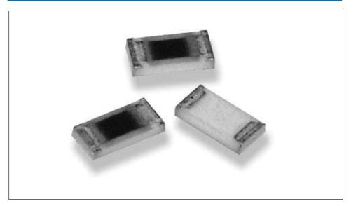
Precious metal terminations are screen printed onto a ceramic base and fired. The resistive element is screen printed and fired and the passivation layer added. Each resistor is trimmed to tolerance by sand blasting. The prescribed tile is broken into strips, the end plating is fired on and the strips broken into individual components. Final termination is made by electroplating.
