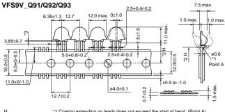
\*1 Coating extending on leads does not exceed the start of bend. (Point A)
