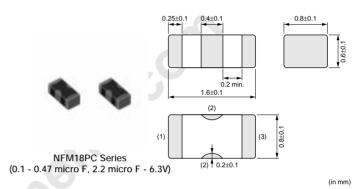
Insulation Resistance Capacitance Rated Voltage Rated Current **Operating Temperature Range** (min.) (M ohm) Part Number (Vdc) (μF) NFM18PC104R1C3 0.1 +20%,-20% 16 2 1000 -55 to +125 NFM18PC224R0J3 0.22 +20%,-20% 6.3 2 1000 -55 to +125 NFM18PC474R0J3 0.47 +20%,-20% -55 to +125 6.3 2 1000 NFM18PC105R0J3 1.0 +20%,-20% 6.3 2 500 -55 to +105 NFM18PC225B0J3 2.2 +20%,-20% 6.3 2 200 -40 to +85 NFM18PC225B1A3 2.2 +20%,-20% 10 4 200 -40 to +85
