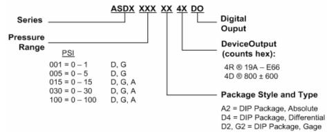
For example: Part #ASDX015A24RD0 = ASDX series, 15 psi absolute, A2 Package, 19A - E66 counts output, digital output
