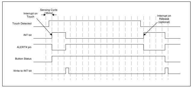
Figure 4.5 Sensor Interrupt Behavior - No Repeat Rate Enabled
