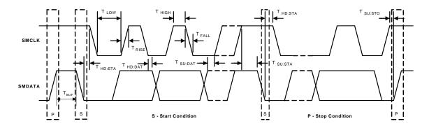
Figure 3.1 SMBus Timing Diagram
