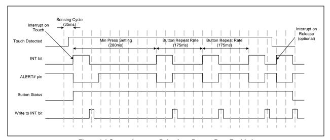
Figure 4.4 Sensor Interrupt Behavior - Repeat Rate Enabled
