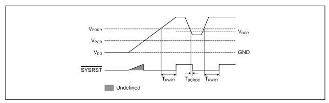
Figure 4.2 POR and PORR With Slow Rising V<sub>DD</sub> and BOR with Falling V<sub>DD</sub>
