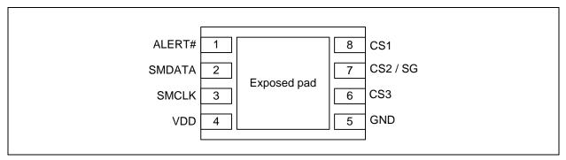
Figure 1.1 CAP1293-1 Pin Diagram (8-Pin 2mm x 3mm TDFN)
