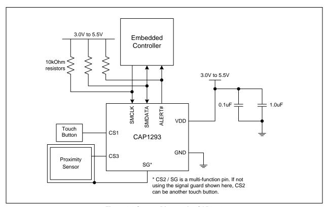
Figure 4.1 System Diagram for CAP1293
