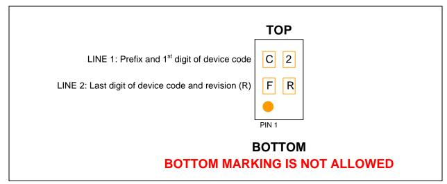
Figure 6.4 CAP1293-1 Package Marking
