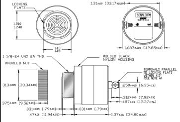
NOTE A: TERMINALS-.032 BRASS TIN PLATED, TAPPED FOR #6-32 SCREW. TWO #6-32 NICKEL PLATED BRASS SCREWS INCLUDED. WILL ACCEPT 1/4' QUICK CONNECT. TE B: MOUNTING- REMOVE BLACK PLASTIC NUT AND INSERT THREADED FRONT THROUGH 1.25' HOLE PUNCHED IN PANEL, IF DRIENTATION IS NEEDED, NOTE LOCKING FLATS ON DRAWING, SCREW NUT BACK ON. DO NOT OVERTIGHTEN.
