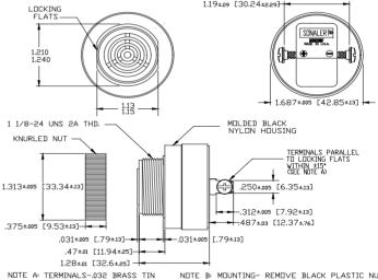
NOTE A: TERMINALS-0.32 BRASS TIN PLATED, TAPPED FOR #6-32 SCREW, TWO #6-32 NICKEL PLATED BRASS SCREWS INCLUDED, WILL ACCEPT 1/4' QUICK CONNECT. MOUNTING- REMOVE BLACK PLASTIC NUT AND INSERT THREADED FRONT THROUGH 125' HOLE PUNCHED IN PANEL, IF DREINTATION IS NEEDED, NOTE LOCKING FLATS ON DRAWING, SCREW NUT BACK ON. DO NOT OVERTIGHTEN.
