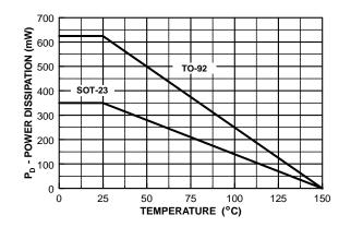
Figure 7. Power Dissipation vs Ambient Temperature
