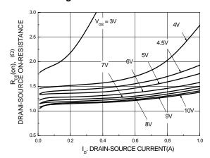
Figure 4. On-Resistance Variation with Gate-Source Voltage
