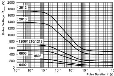
Maximum pulse voltage, single and continuous pulses; applicable if  $\hat{P} \leq \hat{P}_{\text{max}}$ ; for permissible resistance change equivalent to 8000 h operation
