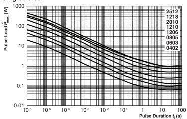
Maximum pulse load, single pulse; applicable if  $\bar{P} \longrightarrow 0$  and n < 1000 and  $\hat{U} \leq \hat{U}_{max}$ ; for permissible resistance change equivalent to 8000 h operation
