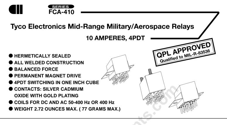
The Series FCA-410 relay is a polarized single-side stable design, where the flux from a permanent magnet provides the armature holding force in the deactivated state, and its flux path is switched and combined with the coil flux in the operated state. This results in appreciably increased contact pressure in both states over that of a spring return nonpolar design. We also manufacture 2-pole and 4-pole versions of this relay.
