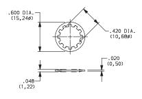
Pushbutton: 8700 Series Rotary: F Series Fits 5/16 Dia. Thread
