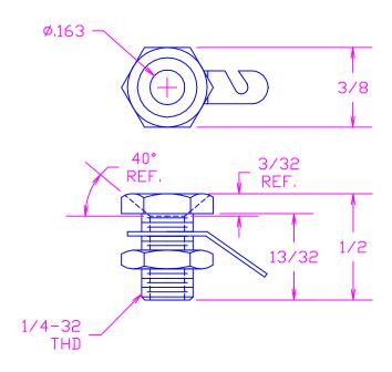
MATERIAL: BODY- BRASS PER ASTM B16,
