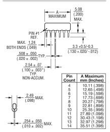
Maximum package length is equal to 2.54 mm (.100") times the number of pins, less .005mm (.002").
