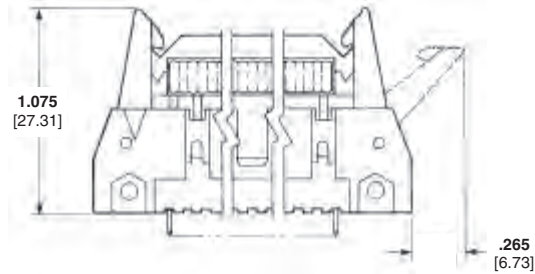
Figure 1 — Use Long Latch for AMP-LATCH Novo Receptacles with Strain Relief & Female Socket Connectors with Strain Relief
