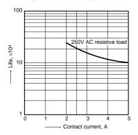
5-(1). Electrical life test (5 A 277 V AC, resistive load) Sample: LKS1aF-12V, 6 pcs. Operation frequency: 20 times/min. (ON/OFF = 1.5s: 1.5s)Ambient temperature: 20°C 68°F
