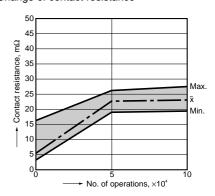
5-(2). Electrical life test (UL lamp load test TV-5)
