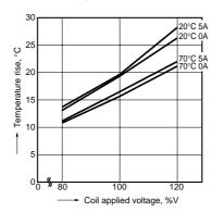
3. Ambient temperature characteristics and coil applied voltage Contact current: 5 A
