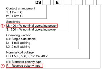
Note: 1 coil latching type are manufactured by lot upon receipt of order. Reverse polarity types available (add suffix-R)
