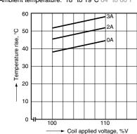
4-(2). Coil temperature rise (2 Form C 2 coil latching type) Tested sample: DS2E-ML2-DC12V Point measured: Inside the coil Ambient temperature: 20° to 21°C 68° to 70°F
